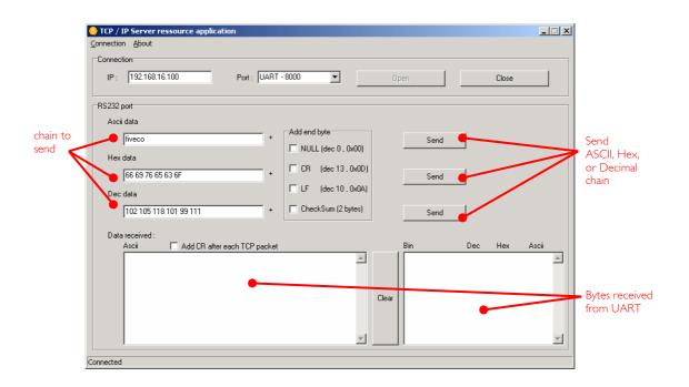
The UART interface is easy to use. Just write the ASCII, HEX or decimal string in the dedicated text box and click corresponding "Send" button. The received bytes are displayed into the "Data received" boxes (same data but different representation).
