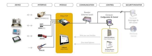
It can be accessed through a TCP socket connection from a computer or through a simple Web Page in a standard browser which can be directly loaded into the device (max 44kb). The module is delivered with a default web page including a Java Applet enabling the controlling of the card.
