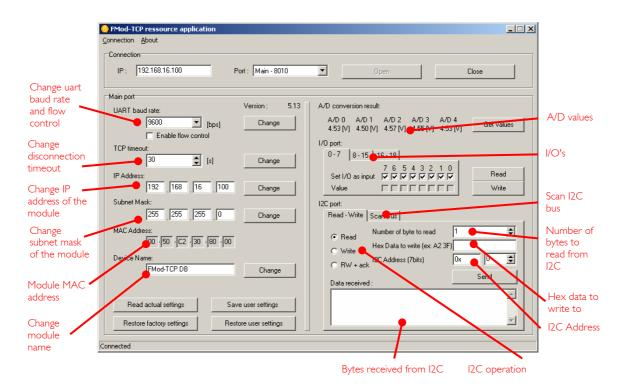
The configuration interface allows the user to change some of the board's settings.
